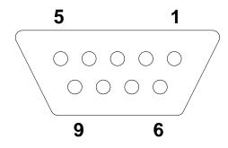
Pin 2: Transmit data Pin 3: Receive data
