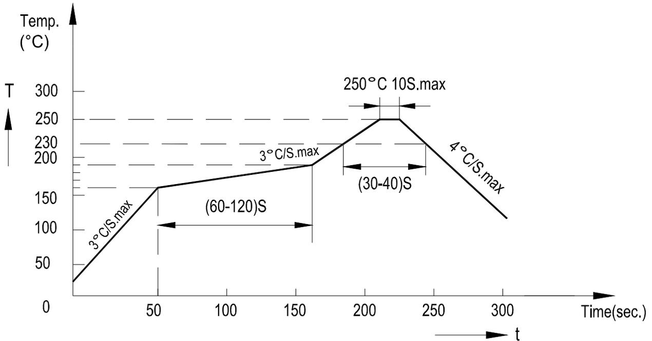
Number of reflow process shall be 2 times or less
