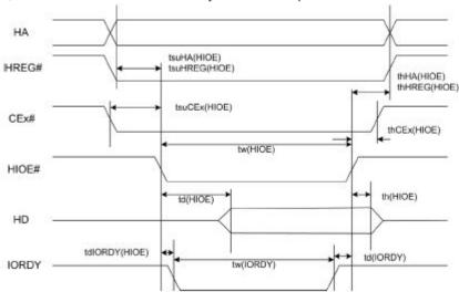
4. I/O Output (Write) Timing Specification
