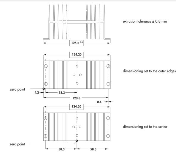
When taking unfavourable extrusion tolerances into consideration, a difference of 0.4 mm arises between the two types of dimensioning with respect to the axis of symmetry.
