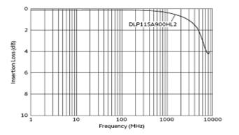
**Differential Mode Transmission Characteristics** (Typical Value)
