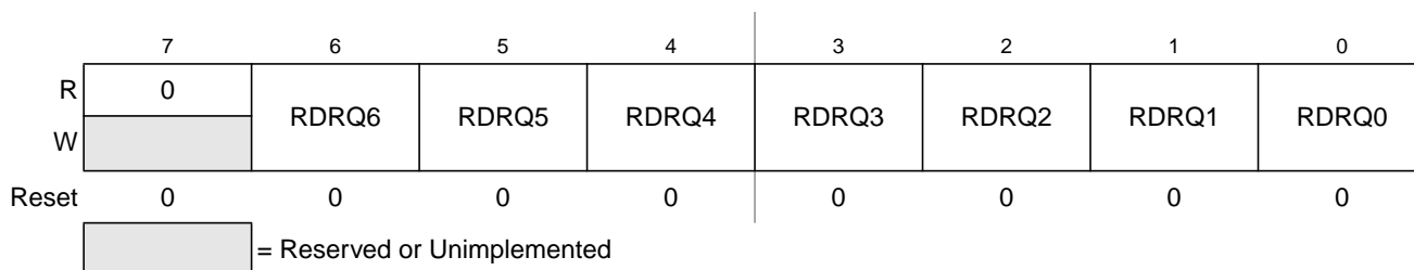
Figure 3-26. Port Q Reduced Drive Register (RDRQ)
