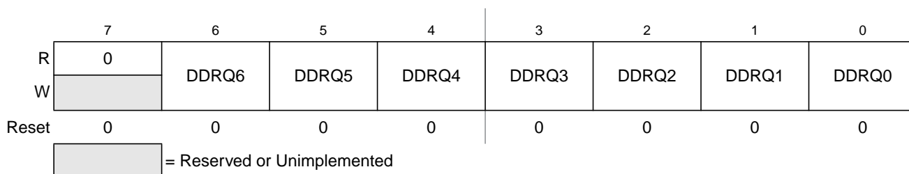
Figure 3-25. Port Q Data Direction Register (DDRQ)
