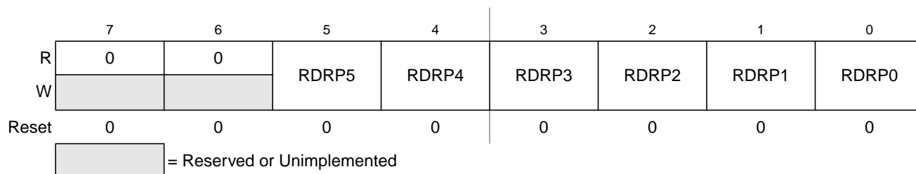
Figure 3-20. Port P Reduced Drive Register (RDRP)
