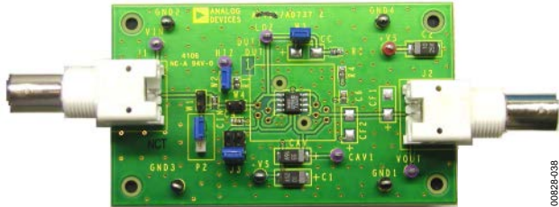
Figure 32. AD737 Evaluation Board
