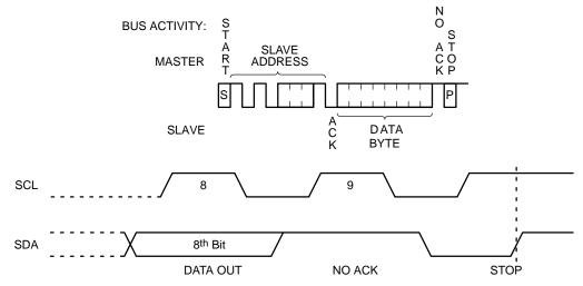
Figure 10. Immediate Read Sequence and Timing
