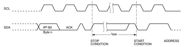
Figure 7. Write Cycle Timing
