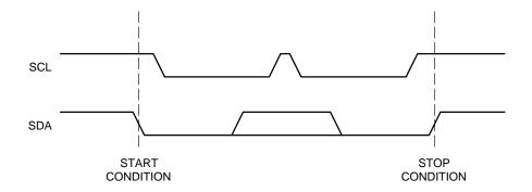
Figure 2. Start/Stop Timing
