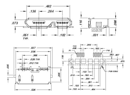
**Description:** USB Socket Micro-B USB 3.0 Surface Mount **Plating Code:** Shell Plating: 10 μ" Gold over 100 μ" Nickel Packaging:
