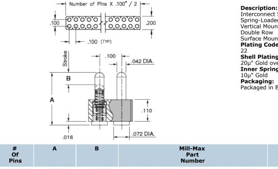
Interconnect SLC Header Spring-Loaded Header Vertical Mount SMT Double Row Surface Mount Plating Code: Shell Plating: 20µ" Gold over 100µ" Nickel Inner Spring Plating: 10µ" Gold Packaging: Packaged in Bulk
