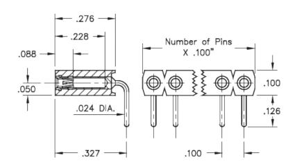
**Description:** Interconnect Socket Right Angle Socket Accepts .025" - .037" (0,635 - 0,94 mm)dia leads Single Row Through Hole Plating Code: **Shell Plating:** 200 μ" Tin (matte finish) over 100
