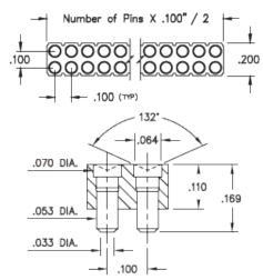
Description: Interconnect Concave Face Target Connector Spring-Loaded Header Vertical Mount SMT Target with Concave Face Double Row Surface Mount Plating Code: 10 Shell Plating: 10 μ" Gold over 100 μ" Nickel Packaging: Packaged in Bulk
