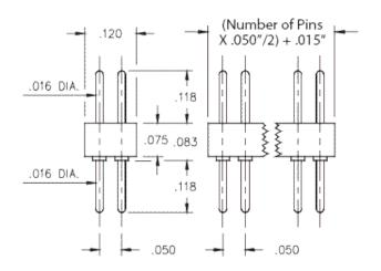
**Description:** Interconnect Header Solder Tail Pin Header .016" (0,41mm) Pin Head Double Row Through Hole
