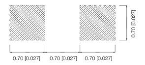
Note: The tolerance unless mentioned is  $\pm$  0.1mm [0.005 in] ; Unit=mm [in]
