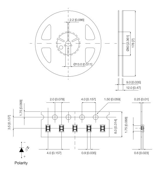
**Note:** The tolerance unless mentioned is  $\pm 0.1$ mm [0.005 in]; Unit=mm [in]
