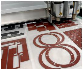
CAD data as a dxf file can be realised directly in ready and zero-toleranced exact cut templates without tooling costs. The outstanding production speed and a cutting technology perfected to the last detail provide an optimal result.
