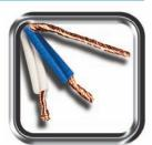
Based on the proven Van Damme 6.00mm Classic Starquad, this miniature version features the same conductors but has a helical lapped copper screen for greater flexibility. Its overall diameter of 4.85mm makes it ideal for bantam adaptor cables, short patch cords and boom microphone cables. The starquad construction ensures excellent rejection of EM and RF interference.
