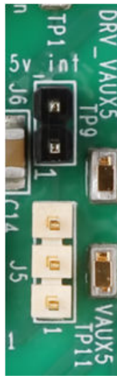
Figure 1-3. Auxiliary 5 VDC Select Jumpers J5 and J6
