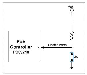
Figure 1-6. I<sup>2</sup>C Bus Test Point and Control Signals
