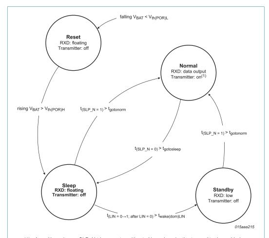
(1) A positive edge on SLP\_N triggers a transition to Normal mode; the transmitter is enabled once TXD goes HIGH; in the event of thermal shut down, the transmitter is disabled.
