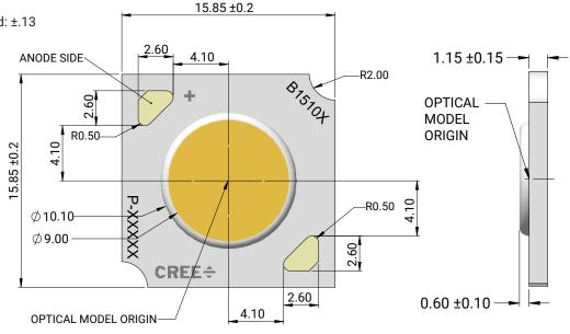
Tc measurement point: either the anode or cathode solder pad
