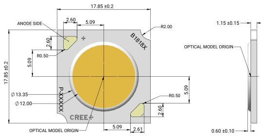
Tc measurement point: either the anode or cathode solder pad
