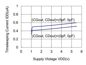
Time Keeping Current vs. Supply Voltage (with no 32K clock output)
