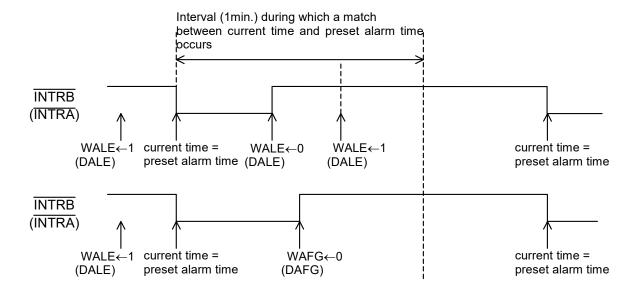
After setting WALE(DALW) to 0, Alarm registers is set to current time, and WALE(DALE) is set to 1, INTRB or INTRA will be not driven to "L" immediately, INTRB or INTRA will be driven to "L" at next alarm setting time.
