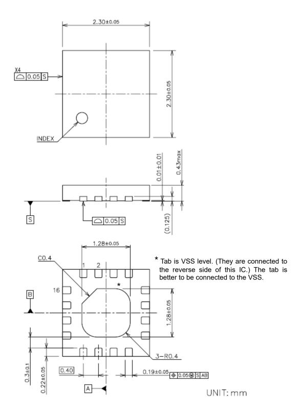
X The side of the all terminals have no plating treatment. Therefore, it may not be able to form solder fillet on the side of the terminals.
