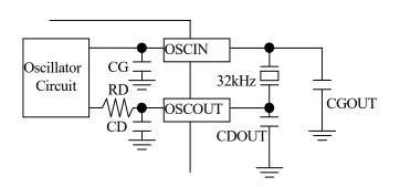
\*1) The CGOUT or/and CDOUT should have a capacitance ranging from 0 to 6 pF.
