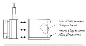
to gain access to the signal board, remove the two Allen-Head Screws and remove rear cover.
