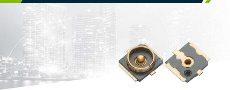
Part of the Taoglas TXR<sup>™</sup> Series of receptacles, the TXR<sup>™</sup> 4 RECE.20449.001E.01 is a 3-pad type wire-toboard SMT Receptacle solution that is ultra-small, lightweight and low profile, 1.6mm max. with an operational frequency range of DC to 6 GHz the TXR<sup>™</sup> 4 RECE.20449.001E.01 is gold plated to provide superior performance and allow easy mounting of the male RF connector.
