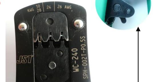
Close the tool lightly until the contact is held (1. Ratchet Lever)
