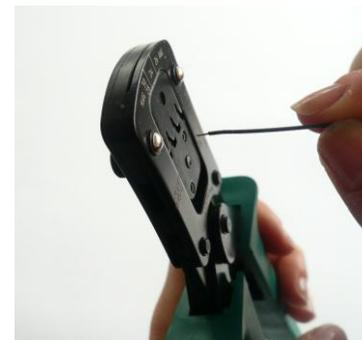
Insert the cable until insulation Stop blade.
