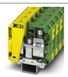
Ground modular terminal block, Connection method: Screw connection, Number of positions: 1, Cross section: 16 mm² - 95 mm², AWG: 4 - 3/0, Width: 20.3 mm, Color: green-yellow, Mounting type: NS 35/7,5, NS 35/15, NS 32
