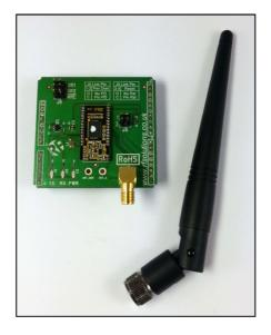
The ZULU*Arduino* provides a radio (Modem) link with easy interface to for upto 2KM range. Range may be further extended with suitable antenna.
