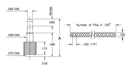
**Description:** Interconnect SLC Header Spring-Loaded Header Vertical Mount SMT Single Row Surface Mount **Plating Code:** Shell Plating: 20μ" Gold over 100μ" Nickel Inner Spring Plating: 10µ" Gold
