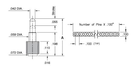
**Description:** Interconnect SLC Header Spring-Loaded Header Vertical Mount SMT Single Row Surface Mount **Plating Code:** Shell Plating:
