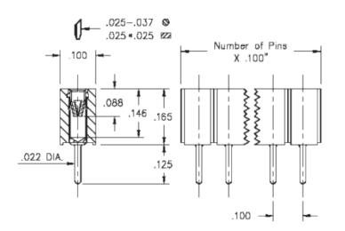
Standard Solder Tail Socket Accepts .025"- .037" (0,635 - 0,94 mm)dia leads Single Row Through Hole Plating Code: 93 Shell Plating: 200 μ" Tin/Lead(93/7) over 100 μ" Nickel Inner Contact Plating:
