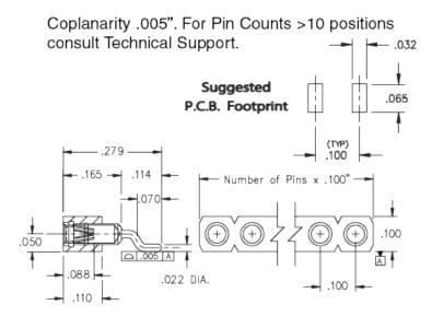
**Description:** Interconnect Socket Horizontal Mount Socket Accepts .025" - .037" (0,635 - 0,94 mm)dia leads Single Row Surface Mount **Plating Code:** Shell Plating:
