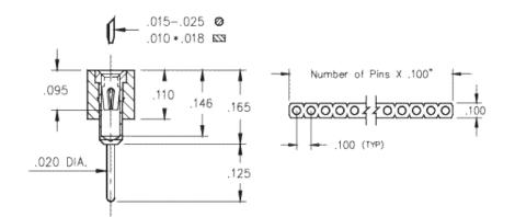
**Description:** Interconnect Socket Standard Solder Tail Socket Accepts .015" - .025" (0,38 - 0,635 mm) dia leads Single Row Through Hole **Plating Code:** Shell Plating:
