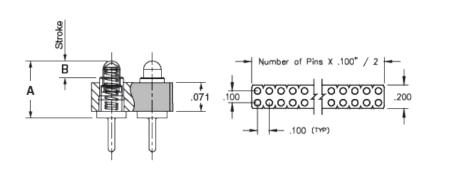
**Description:** Interconnect SLC Header Spring-Loaded Header Vertical Mount Through-Hole Double Row Through Hole Plating Code: 22 Shell Plating: 20µ" Gold over 100µ" Nickel Inner Spring Plating: 10µ" Gold
