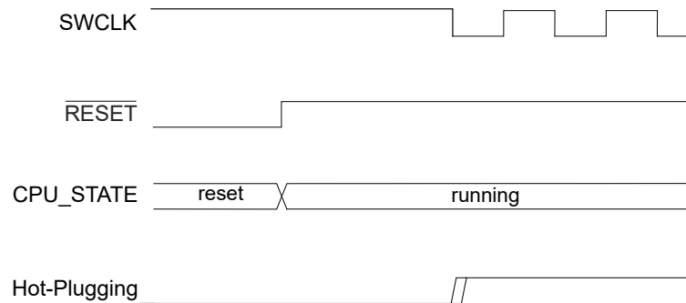
Figure 12-3. Hot-Plugging Detection Timing Diagram
