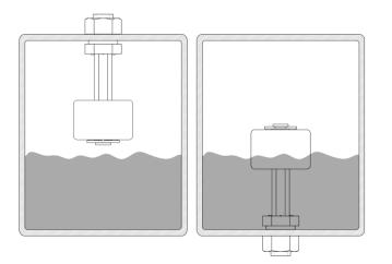
When mounted stem up, operating functions are reversed
