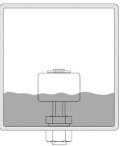
When mounted stem up, operating functions are reversed
