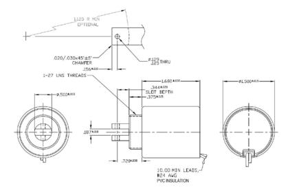
Solenoid shown energized with plunger fully seated Supplied with hex nut shipped loose Spring kits available (consult factory)
