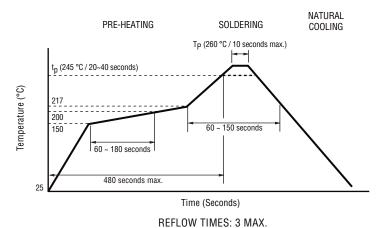
NOTE: 0.12 mm thick solder paste recommended.
