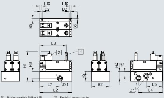
[1] Proximity switch PNP or NPN, size M8x1, plug connection to EN 61076-2-104 [2] Electrical connection to EN 175301-803, type C
