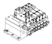
Two 5/2-way single solenoid valves, connected in series, linked via two channels
