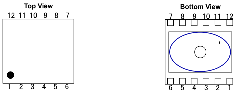
RP605K [DFN(PL)2730-12] Pin Configuration
