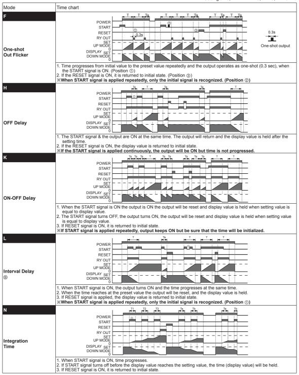
\*\*Initial state: The output is OFF, the display value is "0". (UP mode) The output is OFF and the display value is setting value. (DOWN mode) \*\*When using F output operation modes, if the time is set too short, the output may not work properly. Please set the time at least over 100ms.
