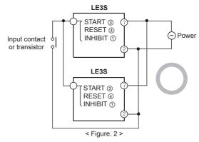
Please use transformer with primary and secondary isolated power for input.
