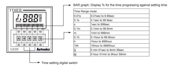
• Setting of operation time: Please select operation time by press the center of 3 ♠, , keys in front panel.
