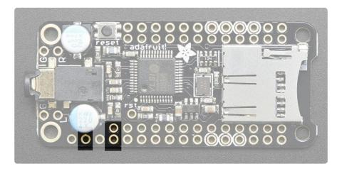
For both headphone & amp version: to power the SD card and MP3 chip, we need power from the 3V (2nd pin) and GND (4th pair of pins).
