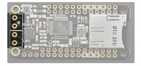
This is the bridge-tied-load output from the VS1053 through the amplifier chip. Connect to 4 to 8 ohm speakers. If you don't need both outputs, just keep one disconnected. Don't connect the outputs together! Nor can you connect the outputs to another amplifier - they are for direct connection to a speaker only!
