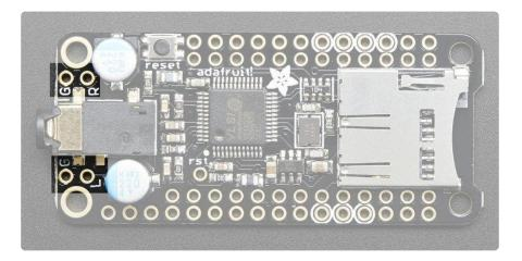
If you don't want to use a 3.5mm jack, you can always connect directly to the Ground, Right and Left pins next to the headphone jack. They are line level, AC coupled outputs - so its safe to connect them to an amplifier or other device input.
