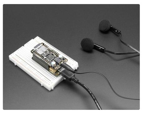
Bend all audio files to your will with the Adafruit Music Maker FeatherWing! It's a funsize version of our <u>Music Maker shield for Arduino</u> (https://adafru.it/tbM)! This powerful shield features the VS1053, an encoding/decoding (codec) chip that can decode a wide variety of audio formats such as MP3, AAC, Ogg Vorbis, WMA, MIDI, FLAC, WAV (PCM and ADPCM). You can do all sorts of stuff with the audio as well such as adjusting bass, treble, and volume digitally.
