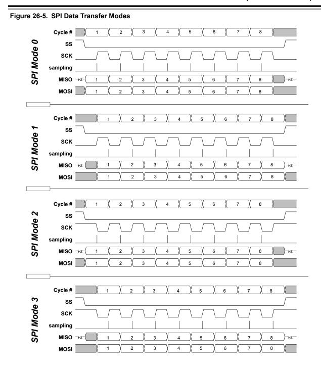
Serial Peripheral Interface (SPI)
