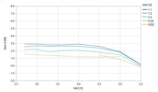
Figure 36-43. Gain Error vs. V<sub>ref</sub> (V<sub>DD</sub>=5.0V, f<sub>ADC</sub>=115 ksps), REFSEL = Internal Reference
