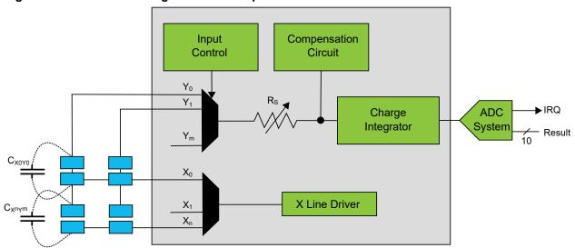
Figure 33-2. PTC Block Diagram Self Capacitance
