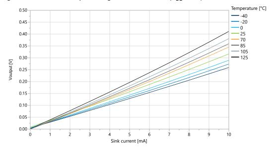
Figure 36-22. I/O Pin Output Voltage vs. Sink Current (V<sub>DD</sub>=5.0V)
