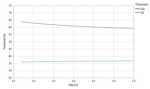
Figure 36-19. I/O Pin Input Threshold Voltage vs.  $V_{DD}$  ( $V_{IH}$ )
