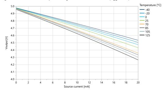
Figure 36-26. I/O Pin Output Voltage vs. Source Current (T=25°C)
