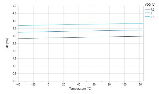
Figure 36-9. Idle Supply Current vs. V<sub>DD</sub> (f=32 KHz OSCULP32K)
