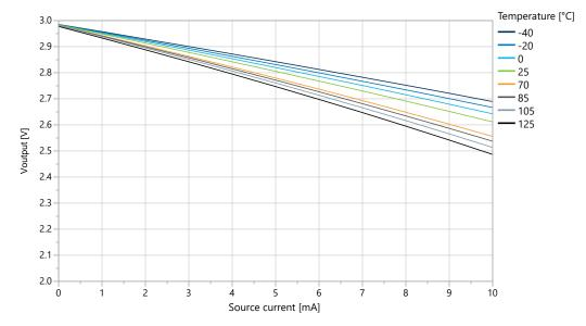
Figure 36-25. I/O Pin Output Voltage vs. Source Current (V<sub>DD</sub>=5.0V)
