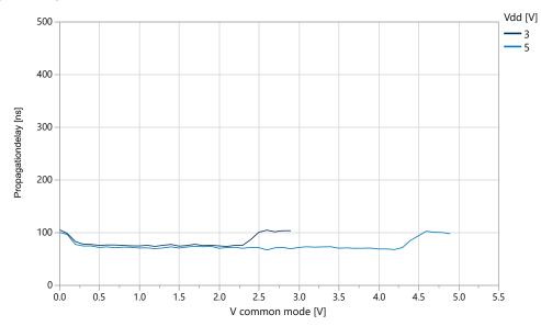
Figure 36-53. Propagationdelay vs.  $V_{CM}$  LPMODE Enabled, Rising Positive input,  $V_{OD}$  = 30mV ( T=25°C)
