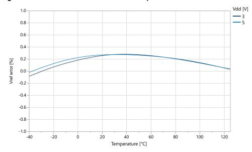
Figure 36-31. Internal 2.5V Reference vs. Temperature
