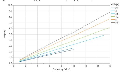
Figure 36-2. Active Supply Current vs. Frequency [0.1, 1.0] MHz at T=25°C
