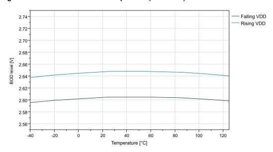
Figure 36-37. BOD Threshold vs. Temperature (Level 4.3V)
