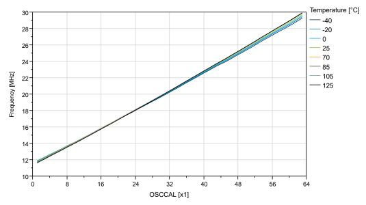
Figure 36-58. OSC20M Internal Oscillator: Frequency vs. Temperature
