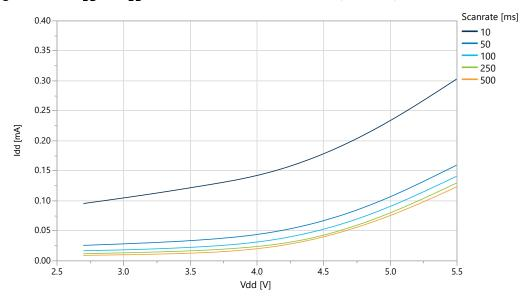
Figure 36-66.  $I_{DD}$  vs  $V_{DD}$  over Scanrates. Filterlevel = 4, T=25°C, Drift cal off.
