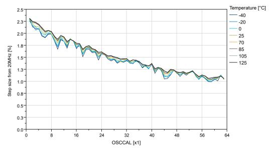
Figure 36-57. OSC20M Internal Oscillator: Frequency vs. Calibration Value (V<sub>DD</sub>=3V)
