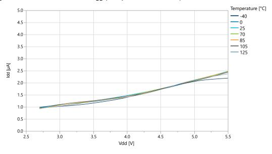
BOD Threshold vs. Temperature Figure 36-36. BOD Threshold vs. Temperature (Level 2.6V)
