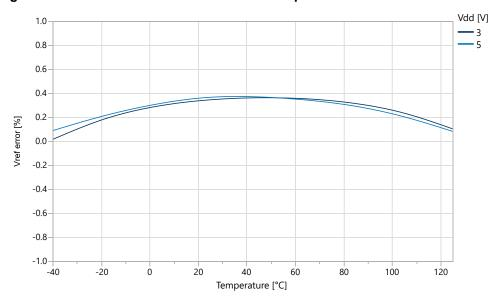
Figure 36-30. Internal 1.1V Reference vs. Temperature
