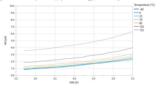
Figure 36-14. Standby Mode Supply Current vs. V<sub>DD</sub> (Sampled BOD Running at 125 Hz)
