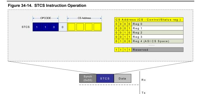
Figure 34-14 shows the data frame transmitted after the SYNCH and instruction frames. There is no response generated from the STCS instruction, as is the case for ST and STS.
