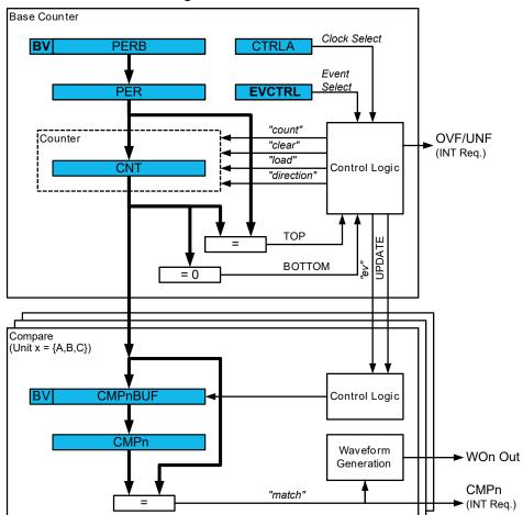
Figure 21-2. Timer/Counter Block Diagram
