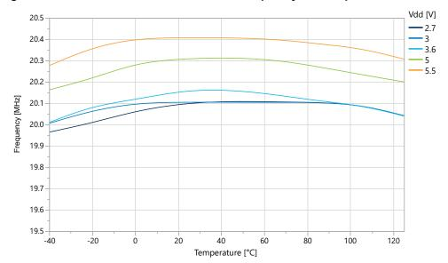
Figure 36-59. OSC20M Internal Oscillator: Frequency vs.  $V_{DD}$
