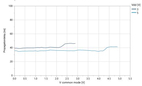
Figure 36-55. Propagation delay vs.  $V_{CM}$  LPMODE Disabled, Rising Positive input,  $V_{OD} = 30 \text{mV}$  ( T=25°C)
