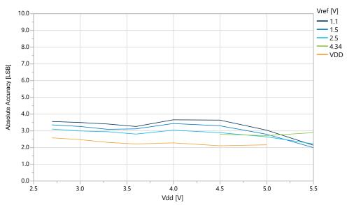
Figure 36-39. Absolute Accuracy vs. V<sub>ref</sub> (V<sub>DD</sub>=5.0V, f<sub>ADC</sub>=115 ksps), REFSEL = Internal Reference
