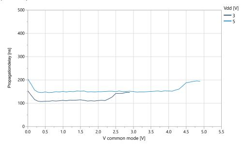
Figure 36-54. Propagationdelay vs.  $V_{CM}$  LPMODE Disabled, Falling Positive input,  $V_{OD}$  = 30mV ( T=25°C)
