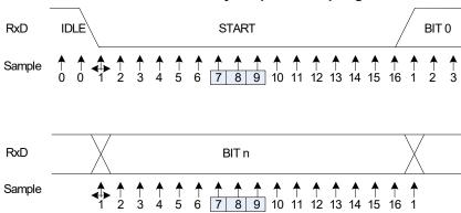
The transmission baud rate must be set up in relation to the selected UPDI clock, which can be adjusted by UPDICLKSEL in UPDI.ASI\_CTRLA. See Table 34-2 for recommended maximum and minimum baud rate settings.
