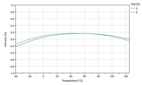
Figure 36-32. Internal 4.3V Reference vs. Temperature
