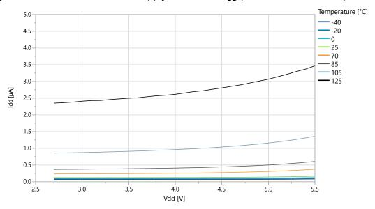
Figure 36-11. Power Down Mode Supply Current vs. V<sub>DD</sub> (All Functions Disabled)
