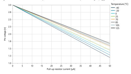
Figure 36-28. I/O Pin Pull-Up Resistor Current vs. Input Voltage (V<sub>DD</sub>=5.0V)
