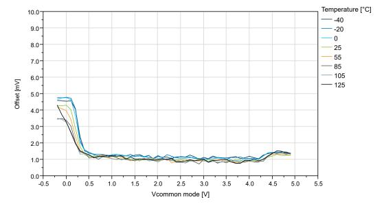
Figure 36-51. Offset vs.  $V_{CM}$  - 10 mV to 50 mV ( $V_{DD}$ =5V, T=25°C)
