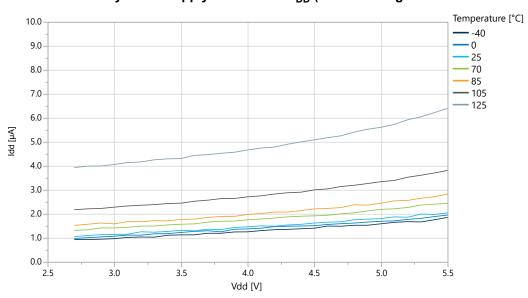
Figure 36-13. Standby Mode Supply Current vs. V<sub>DD</sub> (RTC Running with Internal OSCULP32K)
