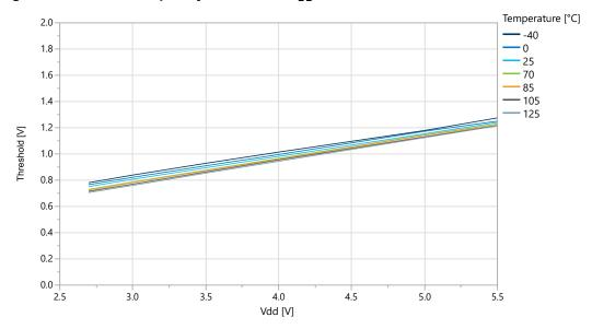
Figure 36-18. I/O Pin Input Threshold Voltage vs. V<sub>DD</sub> (T=25°C)
