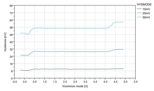
Figure 36-50. Offset vs.  $V_{CM}$  - 10 mV ( $V_{DD}$ =5V)
