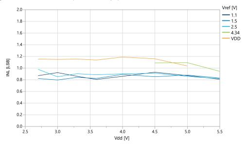
Figure 36-45. INL vs.  $V_{ref}$  ( $V_{DD}$ =5.0V,  $f_{ADC}$ =115 ksps), REFSEL = Internal Reference
