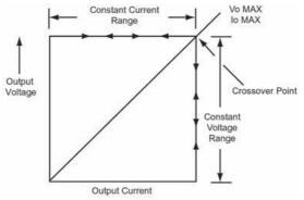
Figure 4 – CC/CV Characteristic
