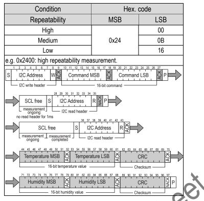
**Table 7:** Measurement commands in single shot mode. The first "SCL free" block indicates a minimal waiting time of 1ms. (Clear blocks are controlled by the microcontroller, grey blocks by the sensor).
