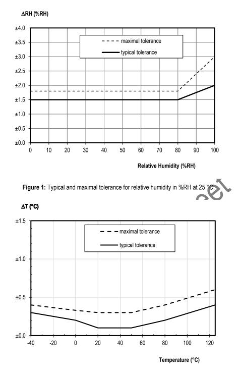
Figure 2: Typical and maximal tolerance for temperature sensor in °C
