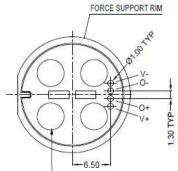
DELICATE SENSOR ELEMENTS INSIDE THE 4 BUMPS PROTRUDING 1.0MM MAX ABOVE RIM, DO NOT APPLY ANY FORCE.
