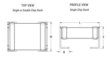
General Information Series KPS SMD Comm X7R Style Stacked Chip SMD, MLCC, Stacked, Single Chip, Temperature Description Stable Features Temperature Stable RoHS Yes Termination Tin AEC-Q200 No Component 160 mg Weight 1210-1 Chip Size 78 Weeks Shelf Life MSL 1
