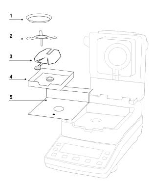
Open heating hood and remove all parts in the right order and clean.
