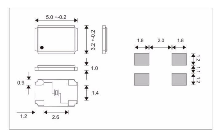
Holder Style Mode Adjustment Tolerance Temperature Stability Operating Temp. Range Load Capacitance ESR Marking 5x32x1 4-Pad Fundamental ± 20PPM at 25°C ± 20 PPM -20°C to +70°C 20 pF 80 Ohm AEL 9.84375 WWYY
