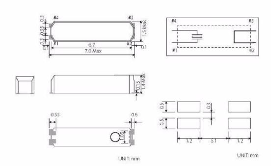
Holder Style Mode Adjustment Tolerance Operating Temp. Range Load Capacitance ESR Static Capacitance (C0) Ageing Marking 7x1,5 SMD Fundamental ± 20PPM at 25°C -40°C to +85°C 7.0 pF 65,000 Ohm Unspecified pF +/-5ppm 1st Year Max AEL32.768
